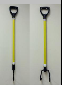
Cable Handling Hooksticks are used in the mining industry as a method of handling energized electrical cables supplying draglines, shovels, drills and other electrical equipment. Cable voltages from 600 V to 35,000 V are safe to handle when using this device.
