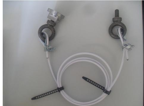
For rip detection two Bulldog units are required one at either side of the conveyor, the BRW belt rip wire connects the two units together by magnetic attachments at each Bulldog. The belt rip wire is placed on the underside of the conveyor approx 25mm down from the bottom of the belt see the figure below.
