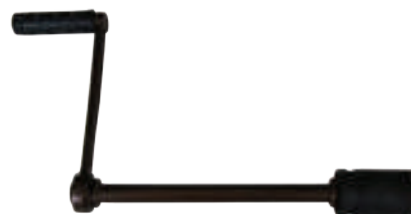
EZ Handle used to fully remove nuts from the stud after loosening the nut.
