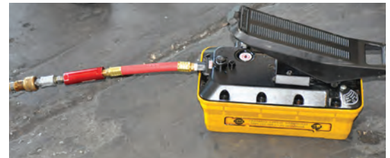
MODEL 10601K being used on ESCO 10500 Hydraulic Pump to regulate air pressure down to the manufacturer suggested 110 psi.
