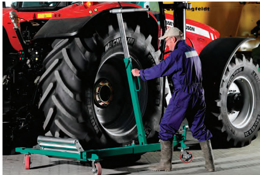
Double Acting Hydraulic System, allowing for hands-free switch between lifting and lowering action for safe and controlled lowering.
