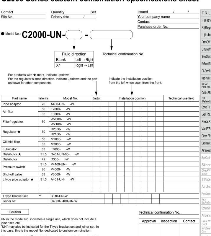
Using pressure switch P□100-UN-W at the end of the combination requires that pipe adaptor A 00-UN-W be added at the end. (The horizontal direction port does not have threads.)
