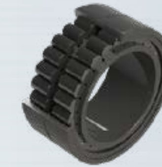
All cylindrical roller bearings with "black oxide" surface treatment to reduce friction and slippage between the rollers and raceways, as well to favor the lubricant film formation.
